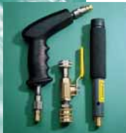
122 spray nozzle, 123 ball valve and 124 foam wand
