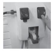
14. To operate button fill units, depress button to dispense product, release button to stop flow. **IF YOU WISH TO LOCK THE BUTTON IN THE "ON" POSITION:** Depress button and slide button lock up, **TO UNLOCK, DE-PRESS BUTTON AND RELEASE.**
