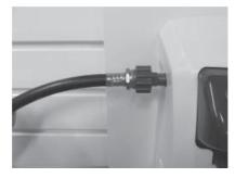
12. Purge air from the system by depressing the buttons briefly. There may be some water discharged from the eductor vents until the air is purged.
