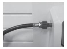
11. Connect water supply hose of at least 3/8" ID to water inlet swivel. Min. 25 psi pressure is required for proper operation, Max. pressure 85 psi and 120°F Max. water temperature. Connect opposite end of hose to water supply. Turn water supply on.
