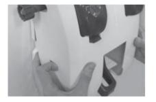
4. Remove the cabinet cover of the unit by pressing the two tabs located on the sides. Rotate up and out on the cabinet cover.
