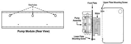
Pump/Motor Assembly-Detached from Pump Module (Side View)
