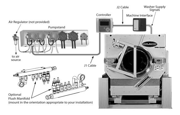
Figure 1 Orion LL-80000 Liquid Laundry Supply Dispenser System Overview
