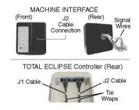
Figure 4 Control Module Connections
