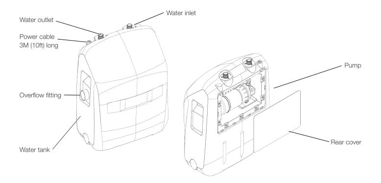
The EvoBoost is designed to supply laundry dispensers (max. 3 low flow EvoClean's) with 2.5 bar (35 psi) consistently. With the EvoBoost installed, chemical delivery will be consistent and extremely accurate, leading to predictable laundry results. The key features of the unit are as follows:
