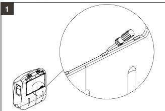
Remove securing clip for pickup tube
