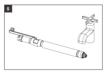
Replace securing clip back onto pickup tube **WARNING TAKE CARE NOT TO DROP THE SECURING CLIP INTO THE WATER TANK**
