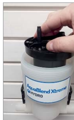
Step 6. Place new motor piston carefully into pump body and replace lid.
