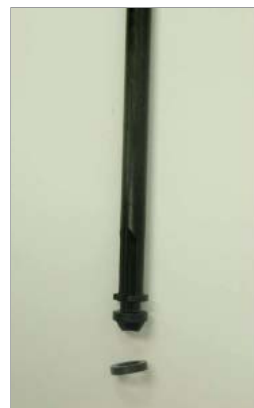
Step 3. Remove shaft with gasket and install new. If damage on sealing surface of shaft, replace shaft.
