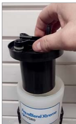
Step 5. Remove motor piston from pump body.
