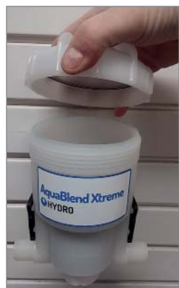
Step 4. Hold body firmly and unscrew the lid. If lid is tight, use 1" (25 mm) socket to loosen.
