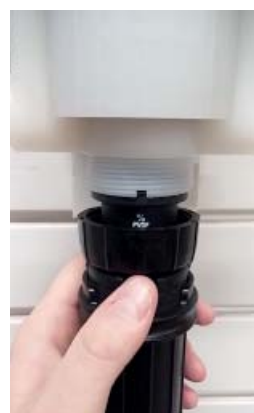
Step 9. Replace lower end assembly and lid onto the pump body. Ensure o-ring is still in the lid before putting it back on.
