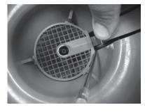
4. Continue lifting screen at each rib location until screen is no longer snapped under ribs.
