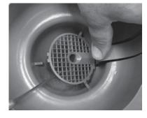
Slide screen off of safety spring and set screen aside.
