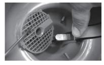
Continue to depress retaining arm to access nozzle (or remove metal safety spring).
