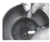
With new nozzle securely in place, locate slot on underside of screen. blank line (If metal safety spring was removed, replace it now.)
