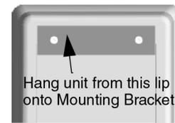
Figure 2 Mounting Bracket
